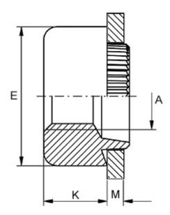
Female thread A = M3,5Height K = 4.0Outer diameter E = 10.0Plate thickness = 0.9 to 1.0
